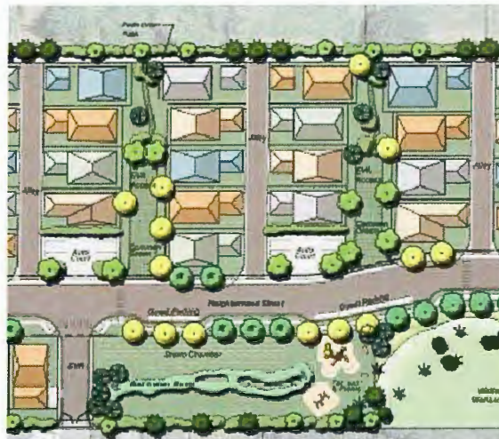
Figure 61 – Site plan for cottages oriented around common greens with alley access for vehicles. Pedestrian connections are provided through common greens and designated pedestrian paths.
