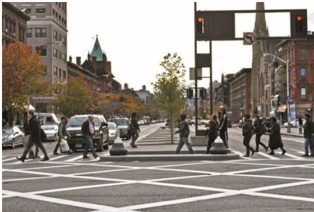
Figure 7: In situations with more than one travel lane in each direction, the pedestrian refuge should be scaled up to match the proportion of space dedicated to vehicles. This creates the added benefit of sufficient space for trees, which further aid in traffic calming and fulfill other urban design goals. (Source: NACTO 5 )
